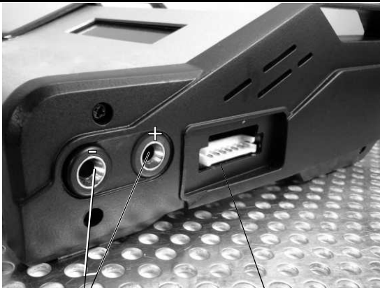
Charge cable sockets red = plus(+) black = minus (-)
